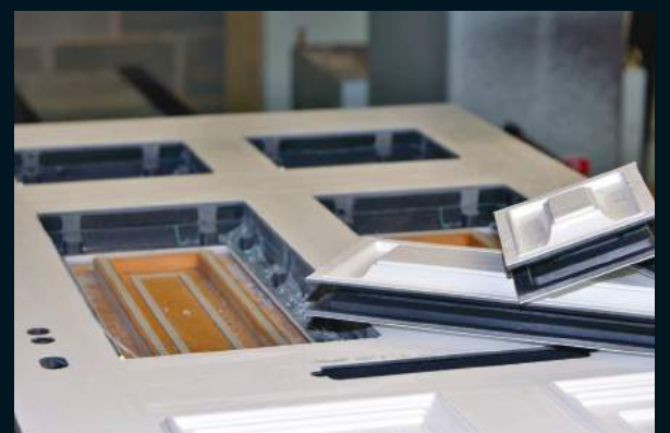
Door after routing operation
